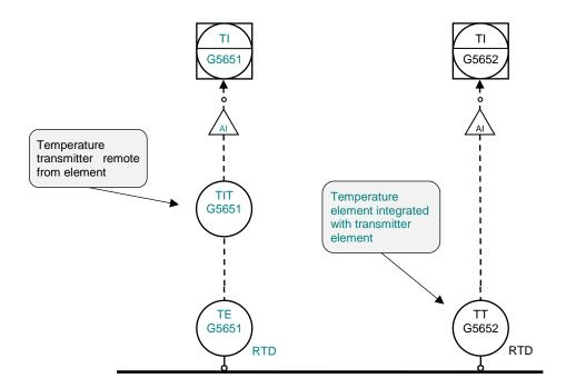
Figure 7-1: Example Temperature Transmitters
