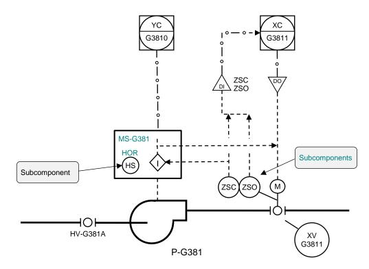
Figure 7-5 : Subcomponents – Electrical and Instrumentation
