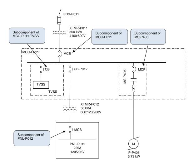
Figure 6-2 : Subcomponents – Electrical Equipment
