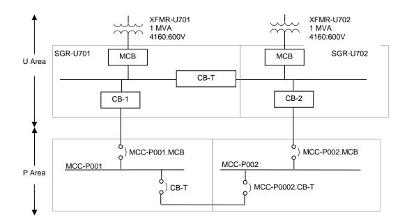
Figure 6-3 : Sample Tie Breaker Identification
