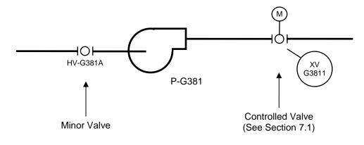
Figure 5-1 : Valve Identification
