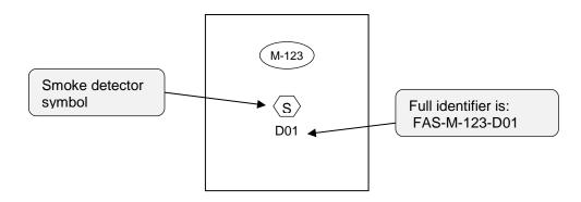
Figure 6-5 : Room Numbering on Drawings – Plan View
