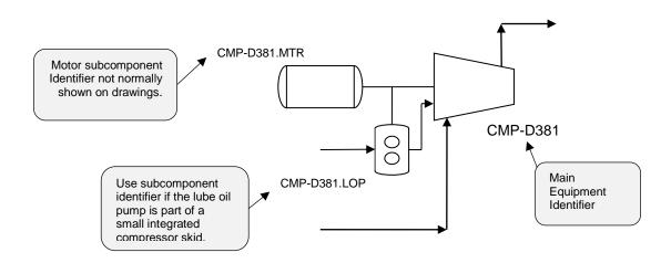
Figure 2-3 : Lube-Oil Pump Subcomponent Example
